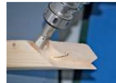
Dovetail at the jack rafter
