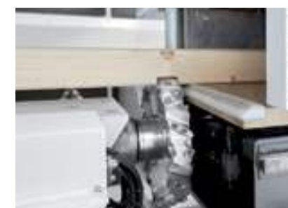
Production of a notch with the routing unit
