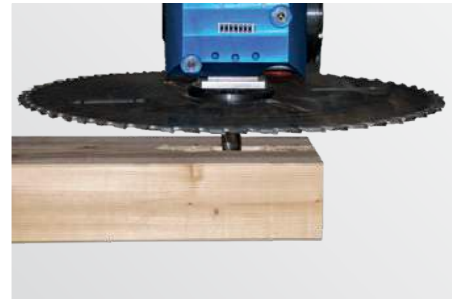
Saw blade with integrated routing unit
