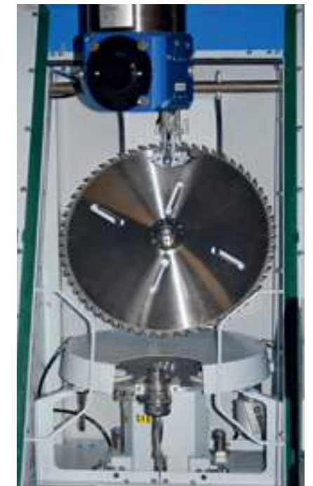
8-slot tool changer with pickup-station
