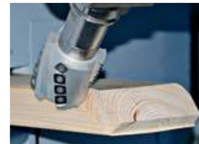
Producing a tenon joint
