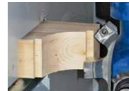
Machining the rafter head
