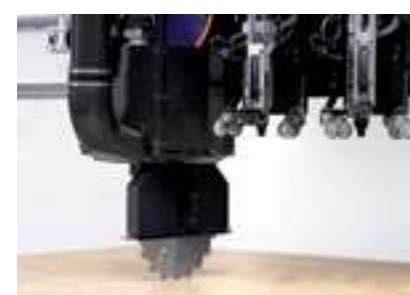
Sawing unit with a built-in protective cover and suction hood
