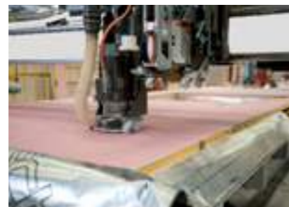
Processing gypsum plasterboard
