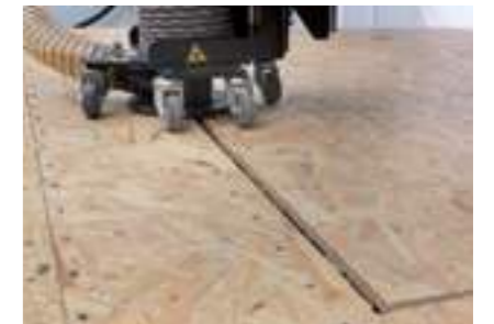
WALLTEQ M-320: fully automatic processing with the routing unit
