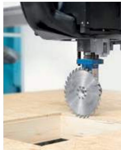
Manufacturing window openings
