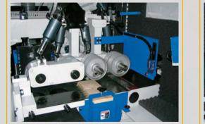
Side Pressure Wheels for Third Spindle
