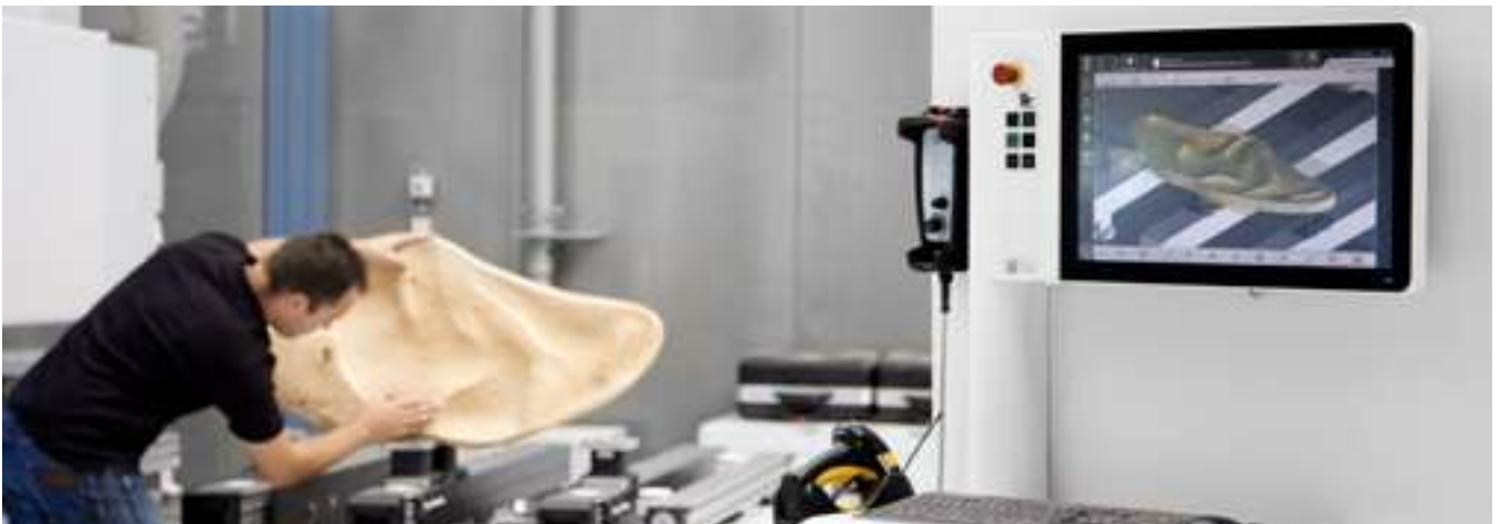
3D scanning and programming of a customer component
