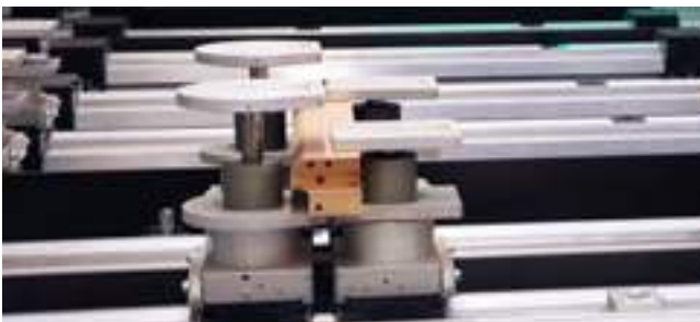
The integrated pneumatic transmission into the clamping elements permits the clamping panels and workpiece surfaces to be cleaned by air jets prior to reclamping. This patented function prevents chip residues from being pressed into the workpiece surface.
