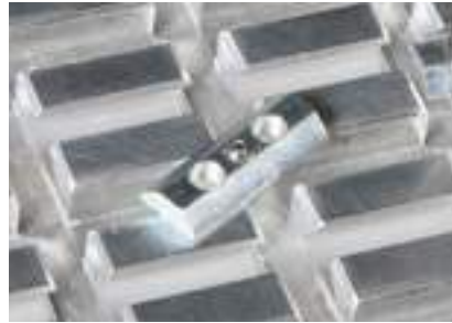
T-nuts, T-slot nut oder slot nut: Slot nuts with thread for positive locking of clamping fixtures in the dovetail guide.
