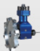
3 Trimming out holes for socket bolts
