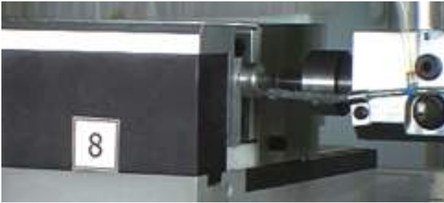
Aluminium thread tapping
