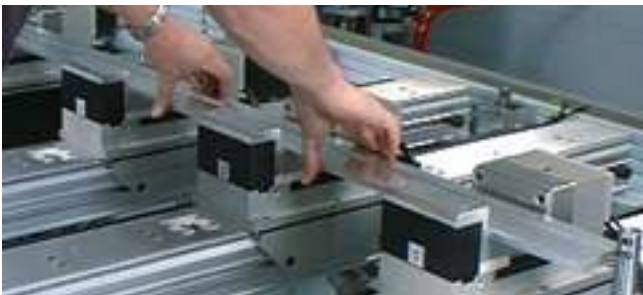
Special clamping elements for aluminium processing
