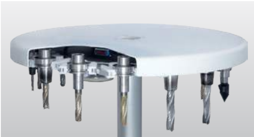
14-fold tool changer moving in X-direction
