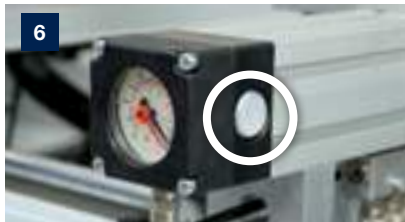
Button for program start Each one button at the left and right hand stop profile act as program start for the processing
