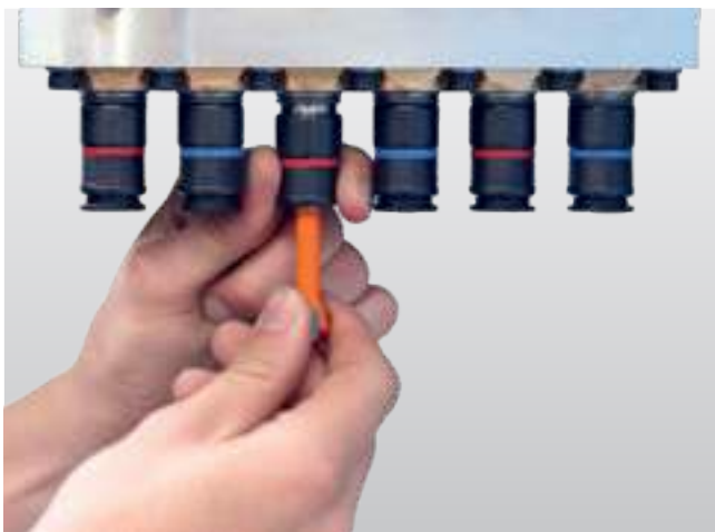
Patented quick-change system for a drill change without tools to reduce setup times.
