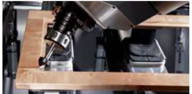
Square corner routing for a glass rebate
