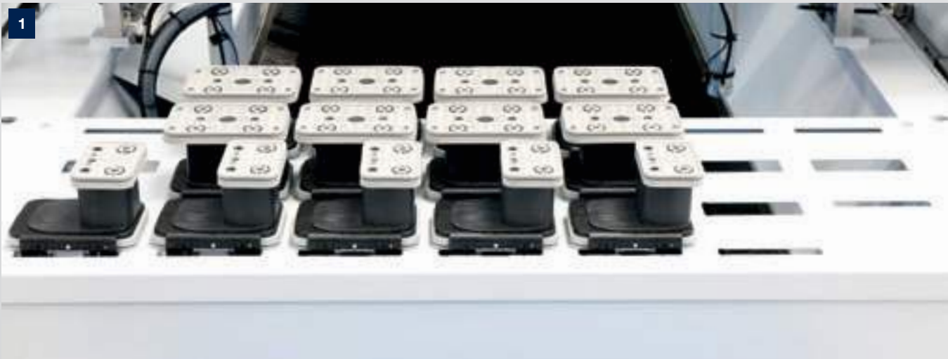
Suction cup storage area Storage area laterally integrated into the machine for vacuum suction cups for easy and fast access
