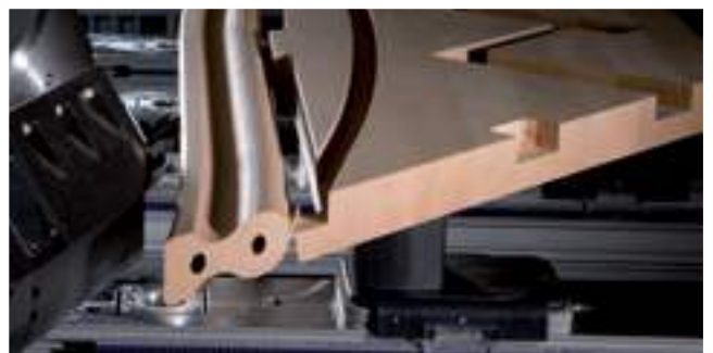
Holes for piling at narrow angles
