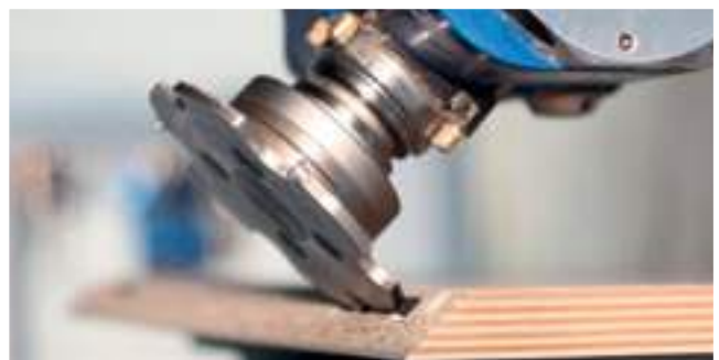
Cutting recesses for connecting fittings
