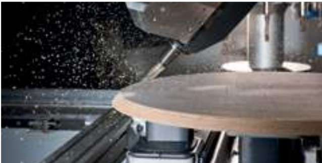
Chamfer trimming on a table top
