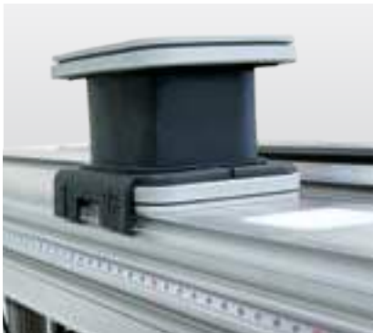
Measuring tape for positioning of suction cups
