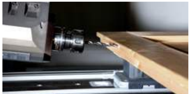
Step drilling for drill-in hinges
