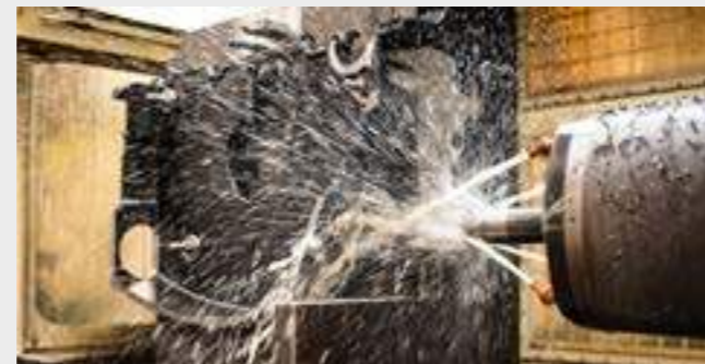
CNC Machining of cast iron saw aggregate
