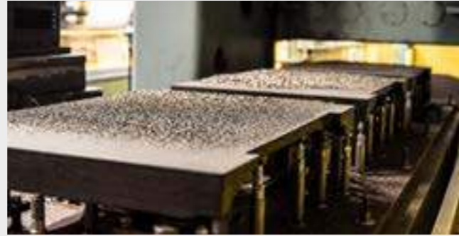
Surface scraping of cast iron table
