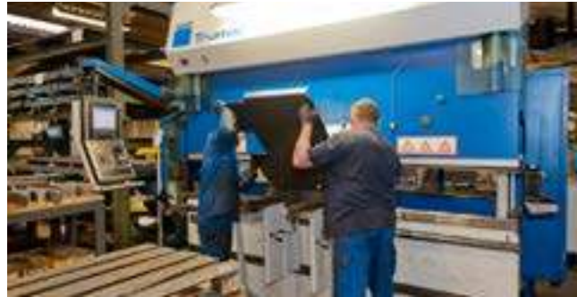
Computer assisted steel plate bending
