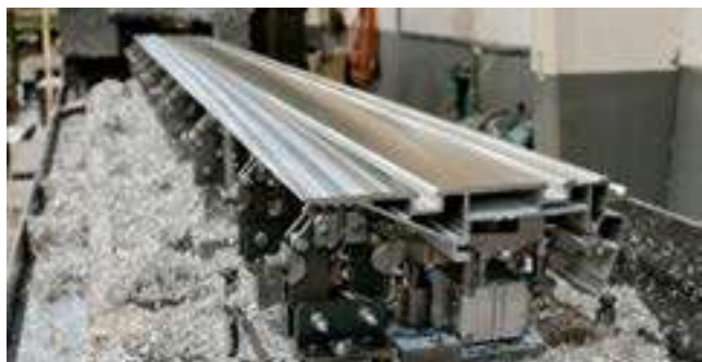
Milling of sliding table surface
