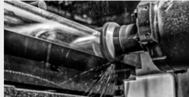
Edge milling of cast iron table
