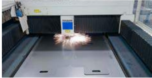
Steel plate laser cutting
