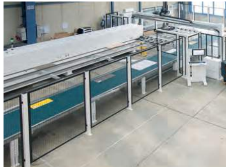
Equipment to achieve CE-conformity: protection grid along the complete return section
