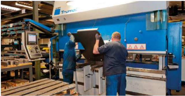
Computer assisted steel plate bending
