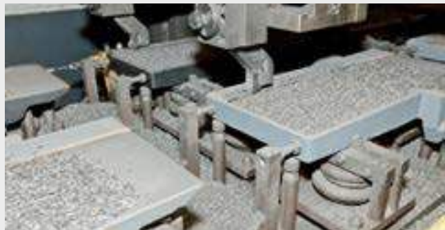
Surface scraping of cast iron table
