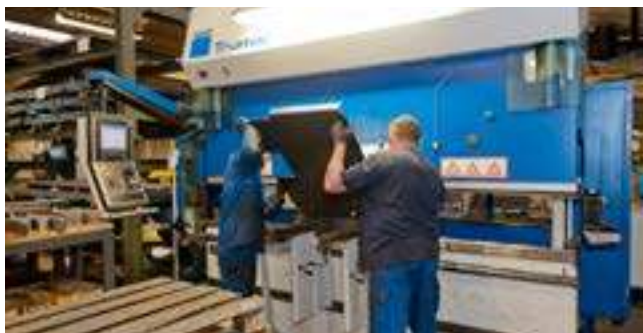
Computer assisted steel plate bending
