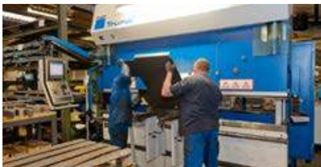
Computer assisted steel plate bending
