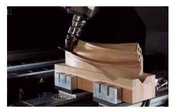
Routing a staircase handrail
