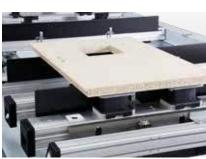
Linear guide and insertion aid - easy handling by consoles with highly precise linear guides and robust insertion aids with two pneumatic cylinders. Vacuum and compressed air connections for pneumatic clamps and clamping templates are integrated in the consoles.
