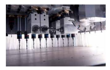
High-speed drilling technology with groove saw
