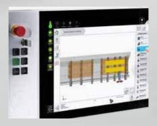
Second operating terminal (option) for optimum shuttle operation without unnecessary walking – ideal for machines with a large work field. Program selection and assignment of the machine is possible on both sides.
