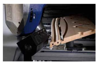
Holes for paling at a tight angle
