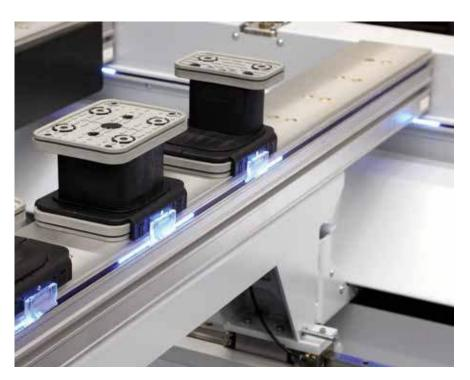
**LED system** – arguably the fastest and safest positioning system for consoles and clamping elements.
