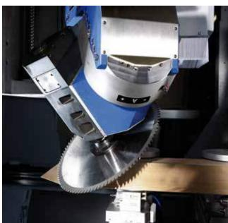
5-axis routing spindle DRIVE5CS/C+ with 10 kW of power (optionally 12 or 15 kW) and a controlled spindle speed from up to 24,000 rpm for a high torque even at low engine speeds.
