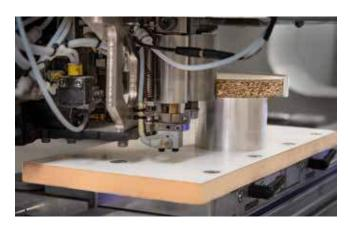
$360^{\circ}$  edge gluing with the powerEdge Pro Duo edge banding unit
