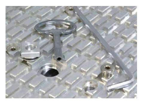
1" vacuum connections with quickopen function by means of switch cabinet key, vacuum openings with precision thread for fixing clamps
