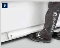
**Switch bar instead of foot switch** – no searching and moving the foot switch – stops, output stroke rails and vacuum clamping can be activated easily.
