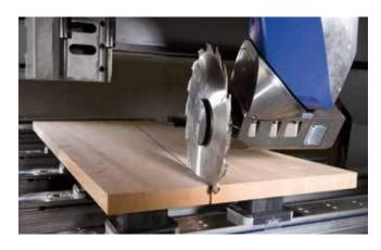
Separating cuts up to 110 mm in height
