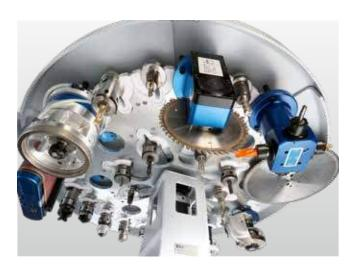
**32-space tool changer** – arrangement of the tools in an inner and an outer ring. For tools and units with a diameter of up to 200 mm and saw blade up to 350 mm in diameter (in the outer ring).
