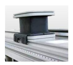
**Measuring tape** for positioning the suction units.
