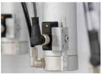
**Electronic cylinder surveillance** Improved safety by electronic surveillance of all stop cylinders
