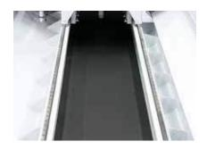
**Chip conveyor** for easy disposal of the offcuts and chips.
