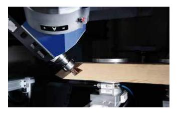
Routing a burr connection for jamb/rail designs
