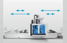
**Dynamic alternating operation** without fixed field subdivision. This means that even in the case of long parts on one side of the machine a short part can still be placed on the other side.
