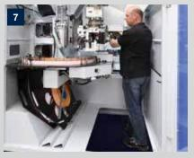
Easy access – drill changes, service, refilling adhesive and edge changes can be carried out easily from the front side of the machine.
