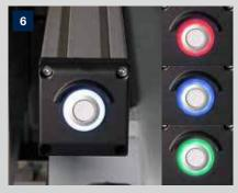
**Button for program start** directly on the left and right stop profile of the machine table. The clamping status is immediately in view thanks to the multi-colored light display.
