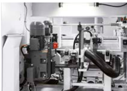
Optional extension for the application of edge sealing or chamfer lacquering
