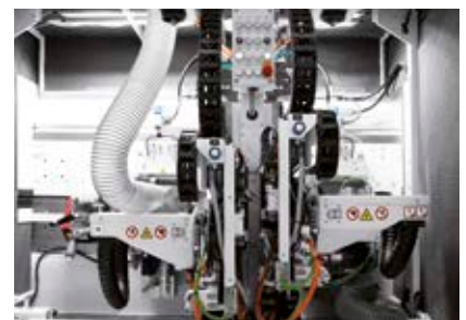
High-power trimming unit SF30 with automatic adjustments
