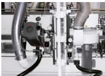
Unit guidance systems with high-precision setting device and swivel-mounted high-frequency motors
