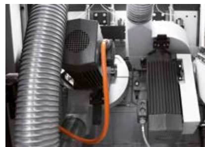
Swivel-mounted high-frequency motors with individual extraction system
