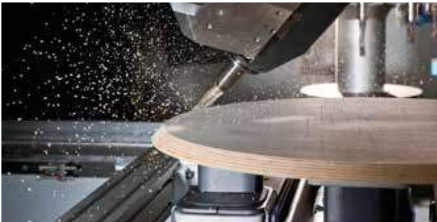
Chamfer cutting on a table top
