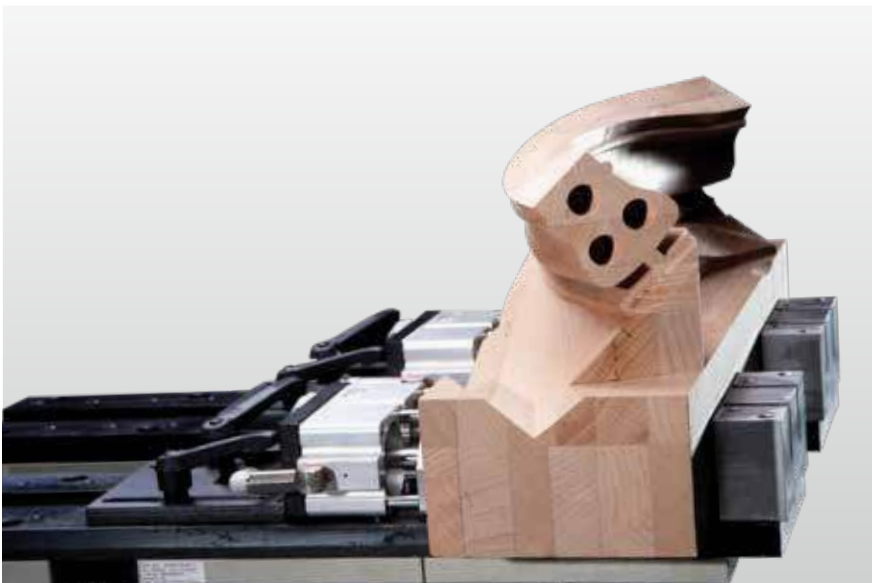
Clamping unit ensures safe and quick clamping of jambs and scantlings.
