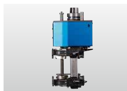
Combined flush trimming and scraper unit for flush trimming and scraper post-processing of the edge profile. The three-sided tracing of the unit balances out workpiece and edge tolerances and guarantees high processing quality incl. tools.
