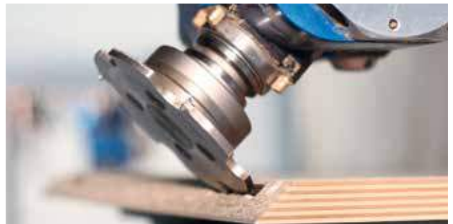
Cutting recesses for connecting fittings
