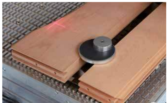
Laser positioning Routing contours can be processed via the cross-laser
