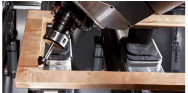
Square corner cutting for a glass rebate
