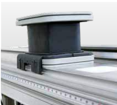
Measuring tape for positioning the suction units.
