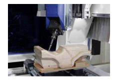
DRIVE5+ five-axis milling spindle:
